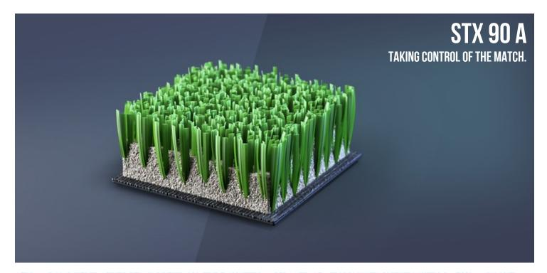
STX 90 A IS A NEXT-GENERATION ARTIFICIAL TURF SYSTEM COMPOSED OF STX MONOFILAMENTS WITH A SEMI-CONCAVE UPRIGHT STRUCTURE AND A CENTRAL SPINE, AND SAND INFILL.
